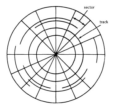
Double-sided, double-density diskettes have either 40 or 80 tracks on each side, and double-sided, high-density diskettes have 80 tracks on each side. Diskettes can have 8, 9, 15, or 18 sectors per track.
